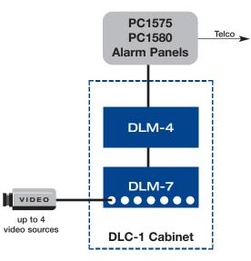
utilizes rotary capture feature of DLM-4 to capture video from up to 4 sources connected to DLM-7
